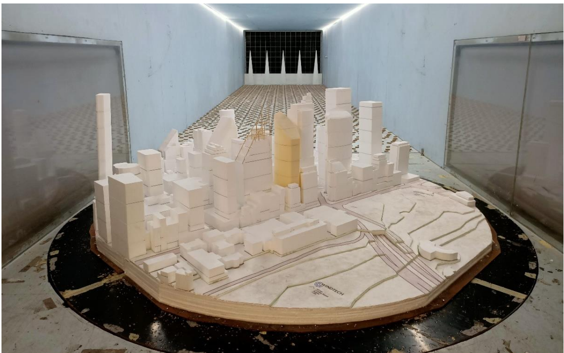
Figure 1f: Photograph of the Wind Tunnel Model (Proposed Envelope, view from the south-east)
