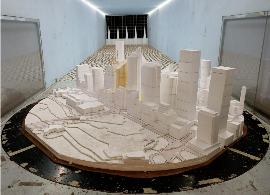
Figure 1b: Photograph of the Wind Tunnel Model (Base Case, view from the north-east)
